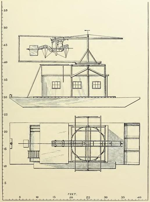
HOUSE-BOAT WITH OVERHEAD LAUNCHING APPARATUS, 1896
